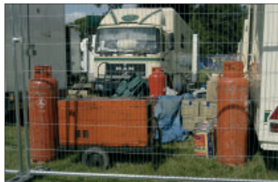
Figure 12: Example of poor storage – LPG cylinders with other combustibles
